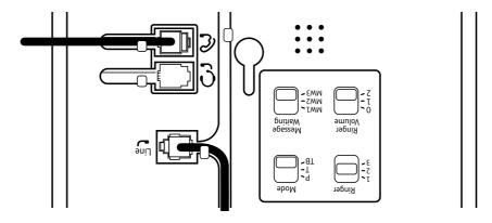
I Plug the other end of the telephone line cord into the wall socket.
